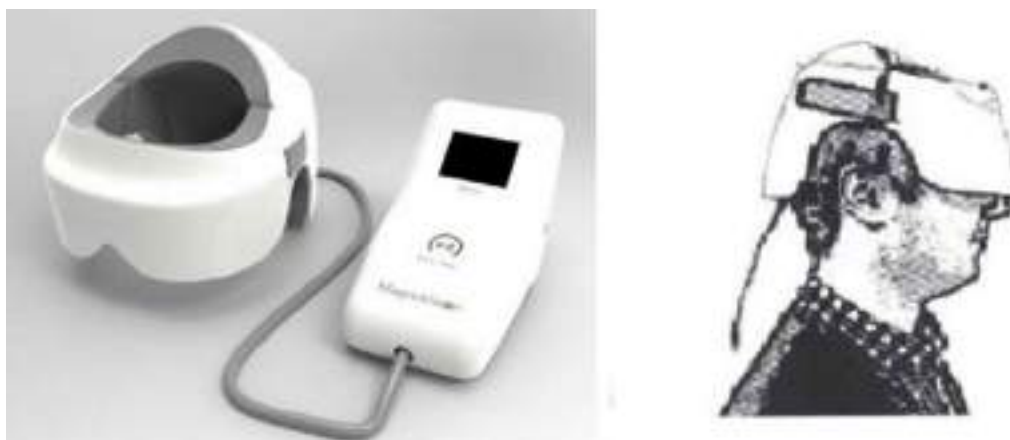
Fig. 2 Retinal electromagnetic stimulator (rEMS) device. Application of the helmet to stimulate the retina-optic nerve and visual pathways [35–37]
